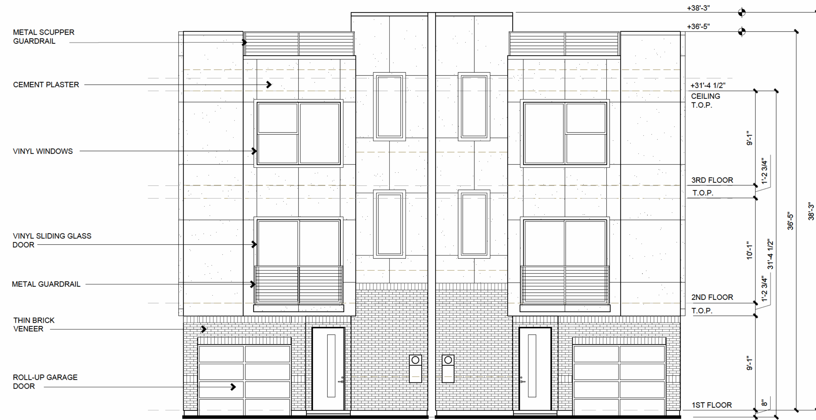
BUILDING 4 (BUILDING 5 SIMILAR) - SOUTH ELEVATION (ALLEY)
